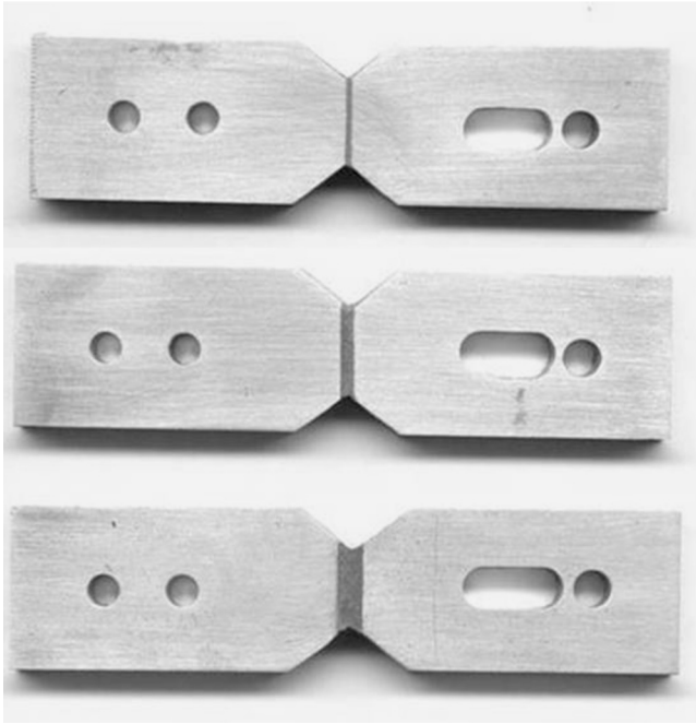
FIGURE 7 Adhesively bonded Iosipescu specimens with three adhesive thicknesses.
