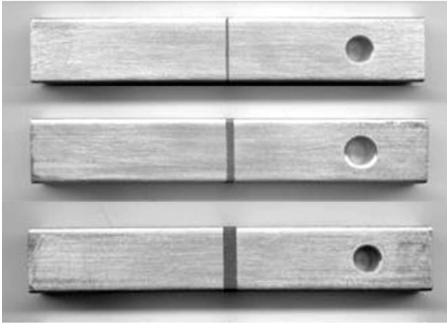
FIGURE 8 Butt-tensile specimens with three adhesive bondline thicknesses.
